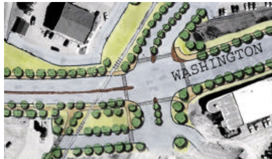
Proposed shared access along Washington Ave. in Kingston creates signalized intersection for left turns.
