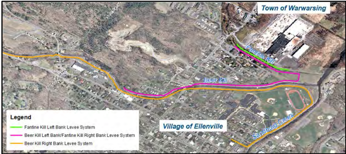
Figure 1: Ellenville FDRP Levee System Alignments
