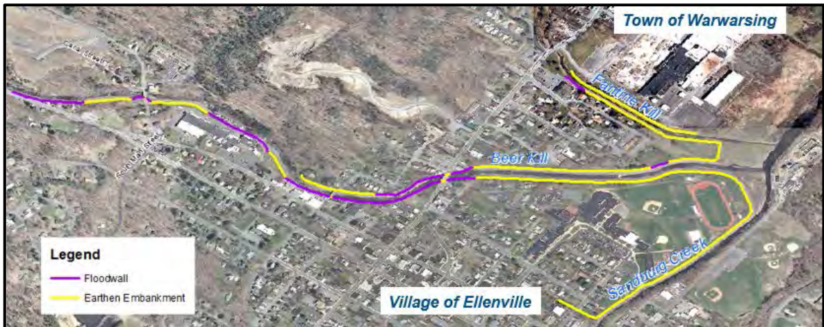
Figure 2: Levee Embankments and Floodwalls
